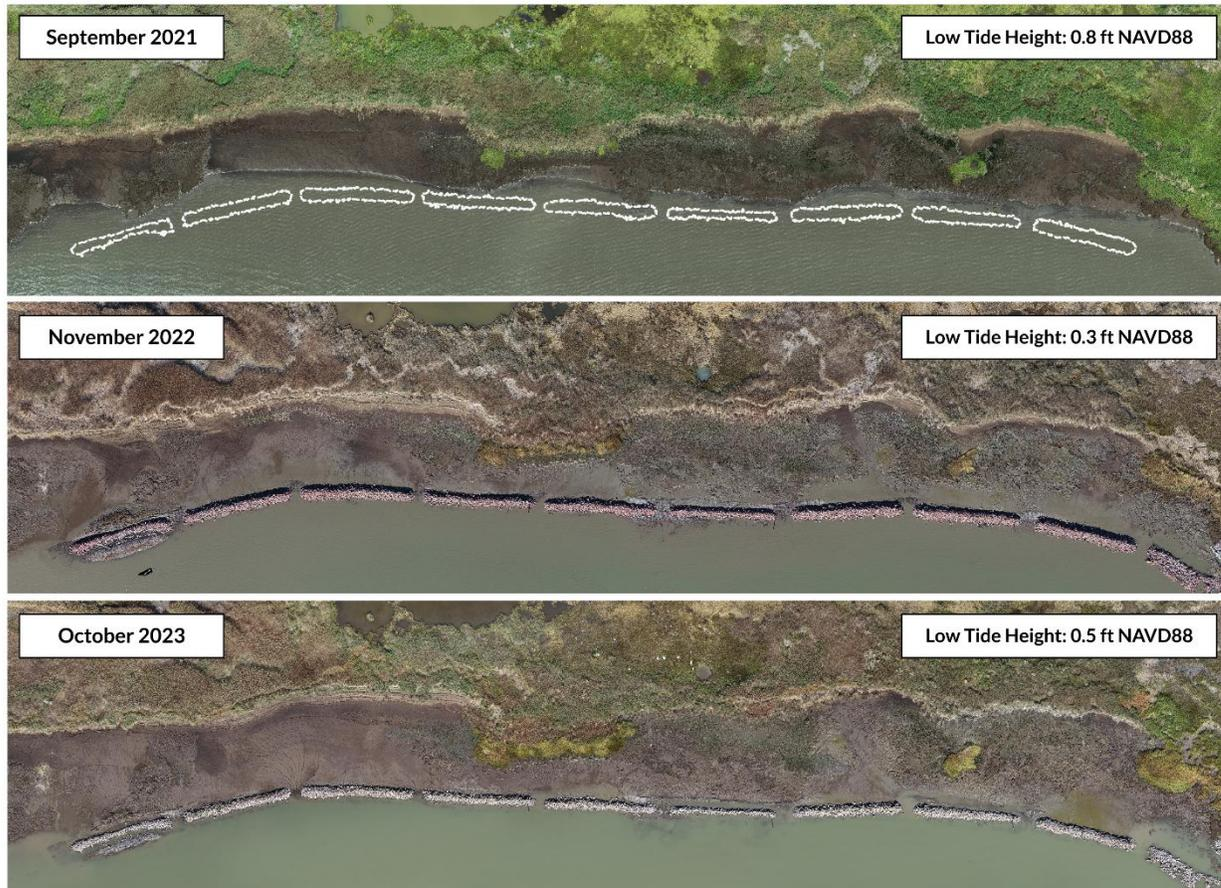
Figure 7: Comparison of the extent of the intertidal zone at low tide from 2021 to 2023. Note that the breakwaters were initially disconnected from the shoreline at first, but sediment accretion has resulted in a low tide shoreline that now reaches the breakwaters.
