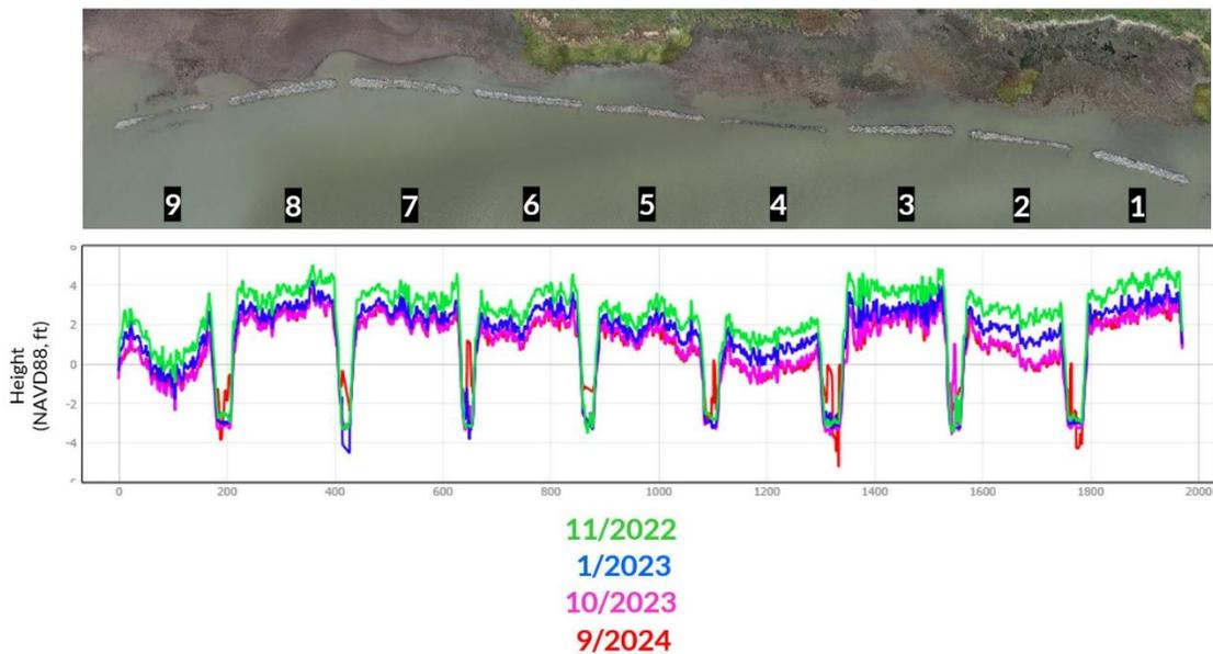
Figure 4: Graph representing a series of drone-based elevation cross sections of the breakwater structures, from west to east. The lines are color-coded according to the time of data capture.
