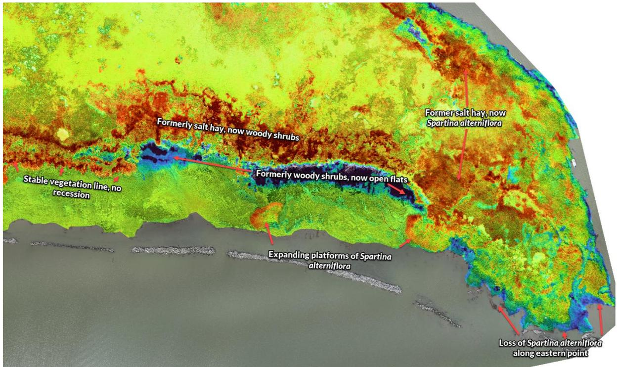
Figure 9: Drone-based digital surface map (DSM) overlaid onto drone imagery of the eastern side of the breakwaters.
