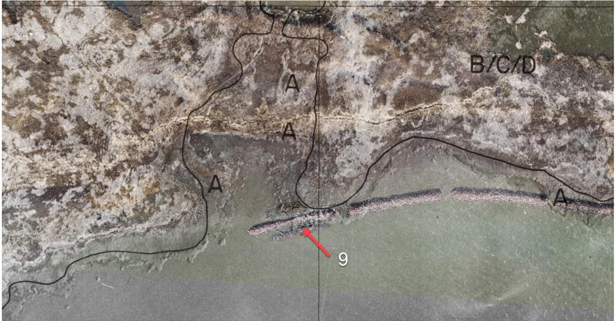
Figure 5: 1977 NJ Wetlands imagery overlaid onto 2023 drone imagery, demonstrating that breakwater 9's significant initial sinking behavior may be related to its position over a former drainage.
