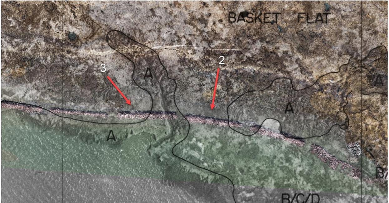
Figure 6: 1977 NJ Wetlands imagery overlaid onto 2023 drone imagery showing that both breakwaters 2 and 3 are positioned over a former drainage.
