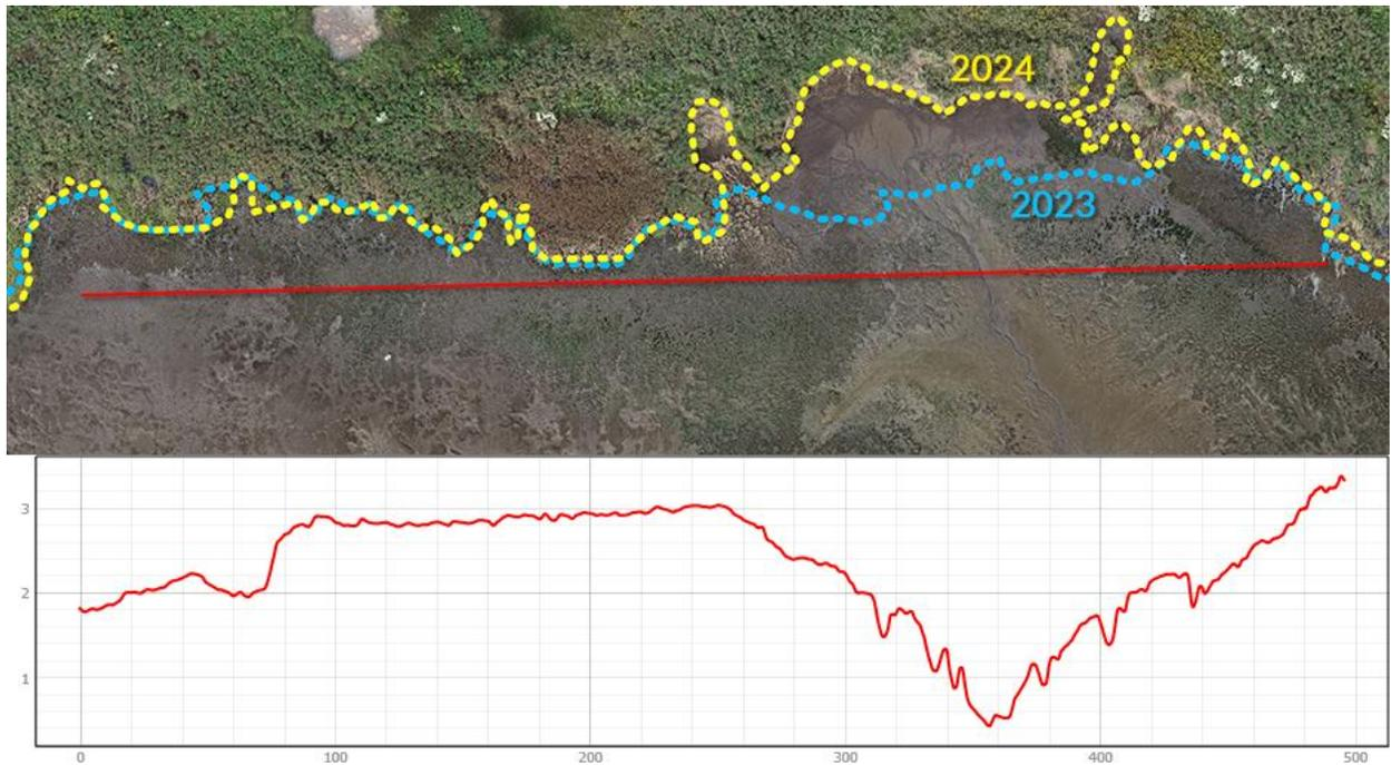
Figure 11: Comparison of the loss of marsh edge with lower elevations in a former drainage cutting through the marsh and intertidal zone.
