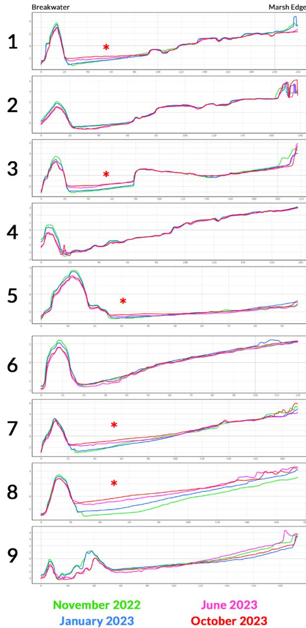
Figure 8: Graphs representing drone-based elevation cross sections from the center of each breakwater to the marsh edge. Breakwaters marked with a red asterisk are those with observable sediment accretion in the landward area behind the breakwaters.
