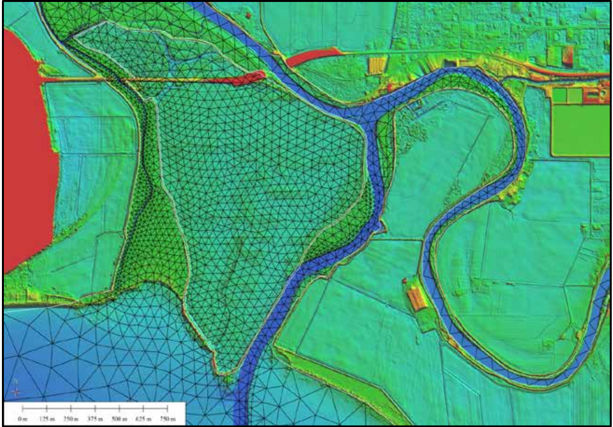
Figure 4-1: (Scenario 0 - Baseline) Model grid overlaying the lidar elevation map
