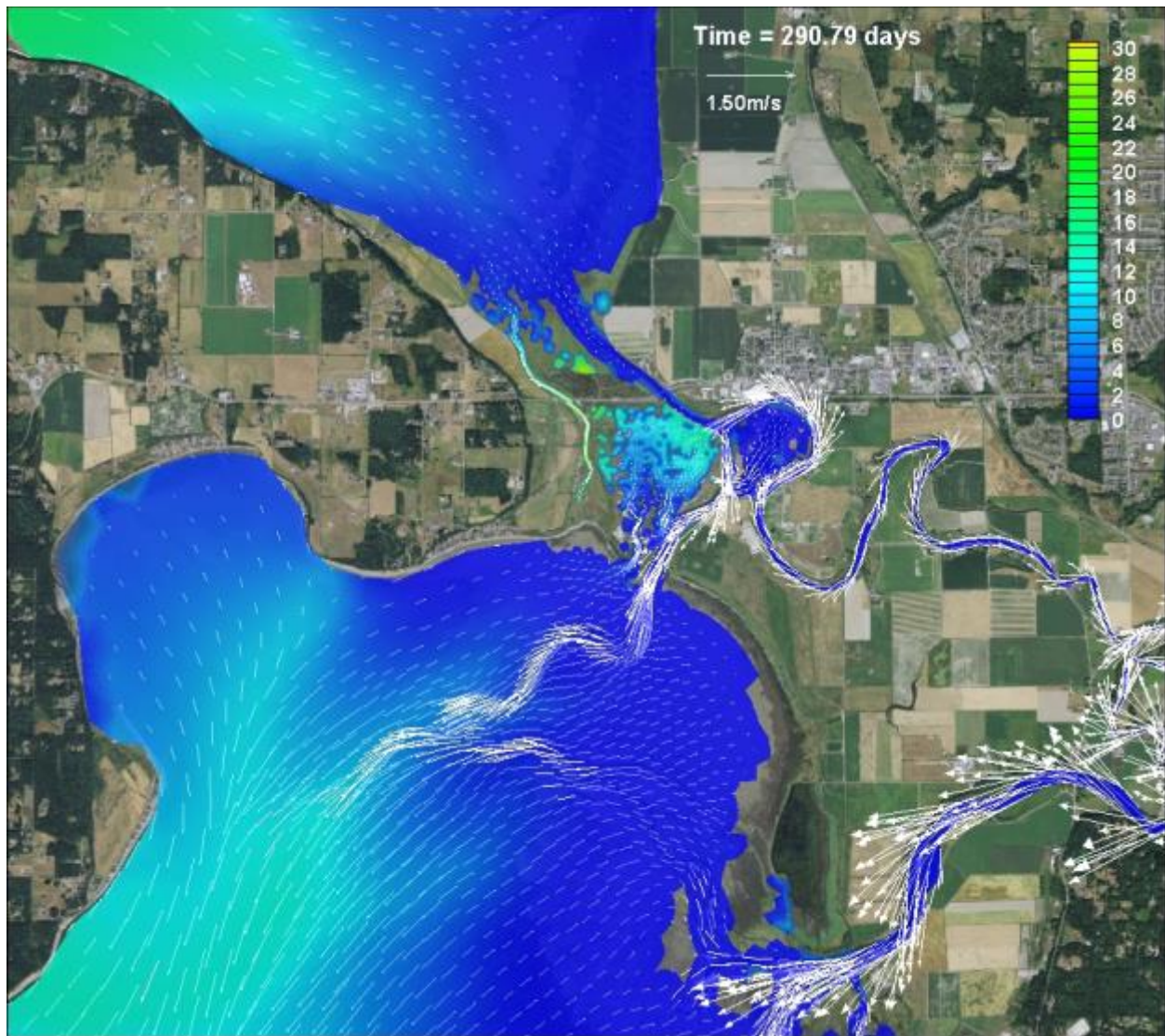
Figure D-27: Scenario 6 (Full Restoration zis a ba + SCN4) – Salinity contours and velocity vectors, high flow (full bank) condition at 26,508 cfs and peak ebb based on October 17, 2005
