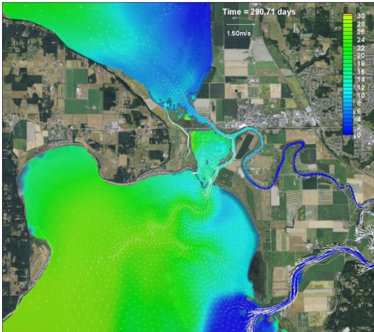
Figure B-9: Scenario 2 (4 Levee Breach Leque) – Salinity contours and velocity vectors, October 17, 2005, high tide
