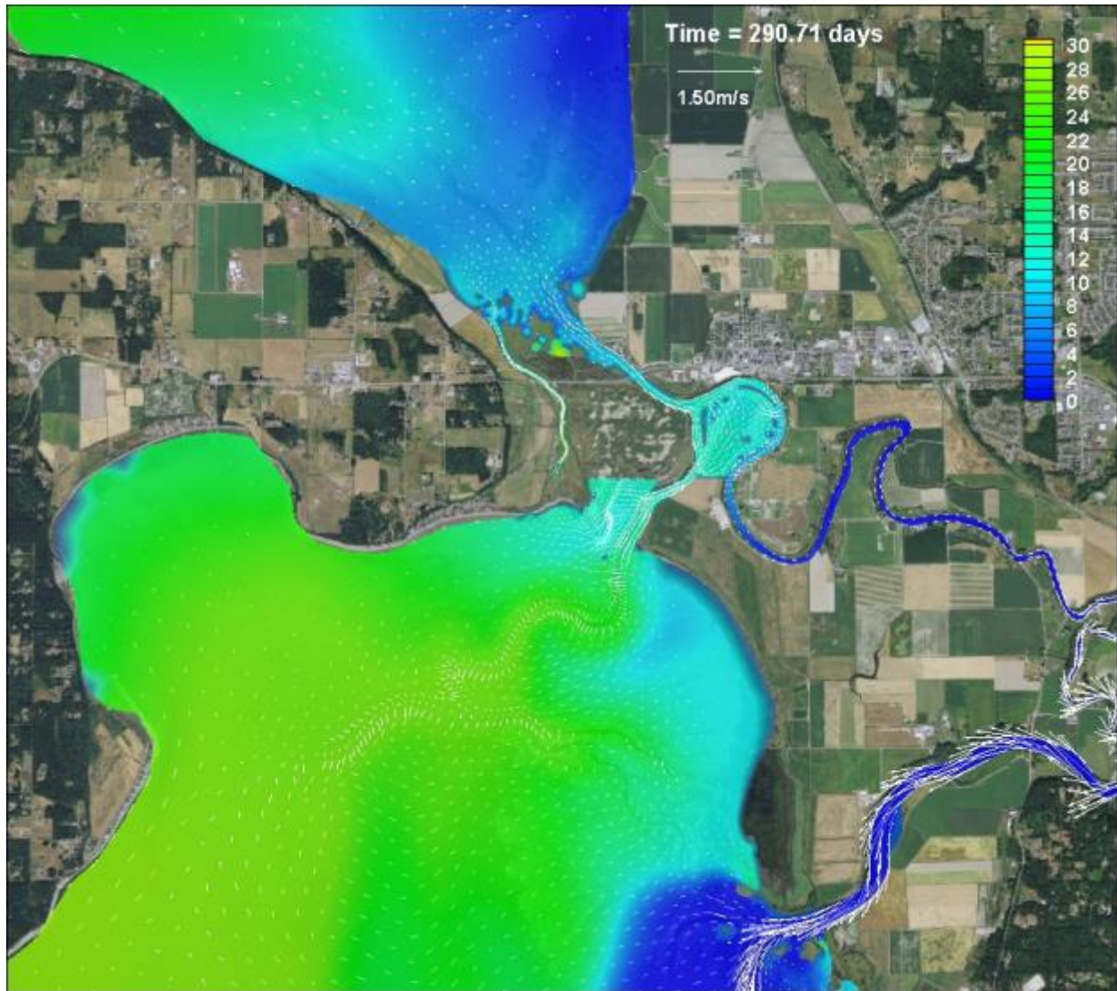
Figure B-21: Scenario 5 (Full Restoration zis a ba + SCN1) – Salinity contours and velocity vectors, October 17, 2005, high tide
