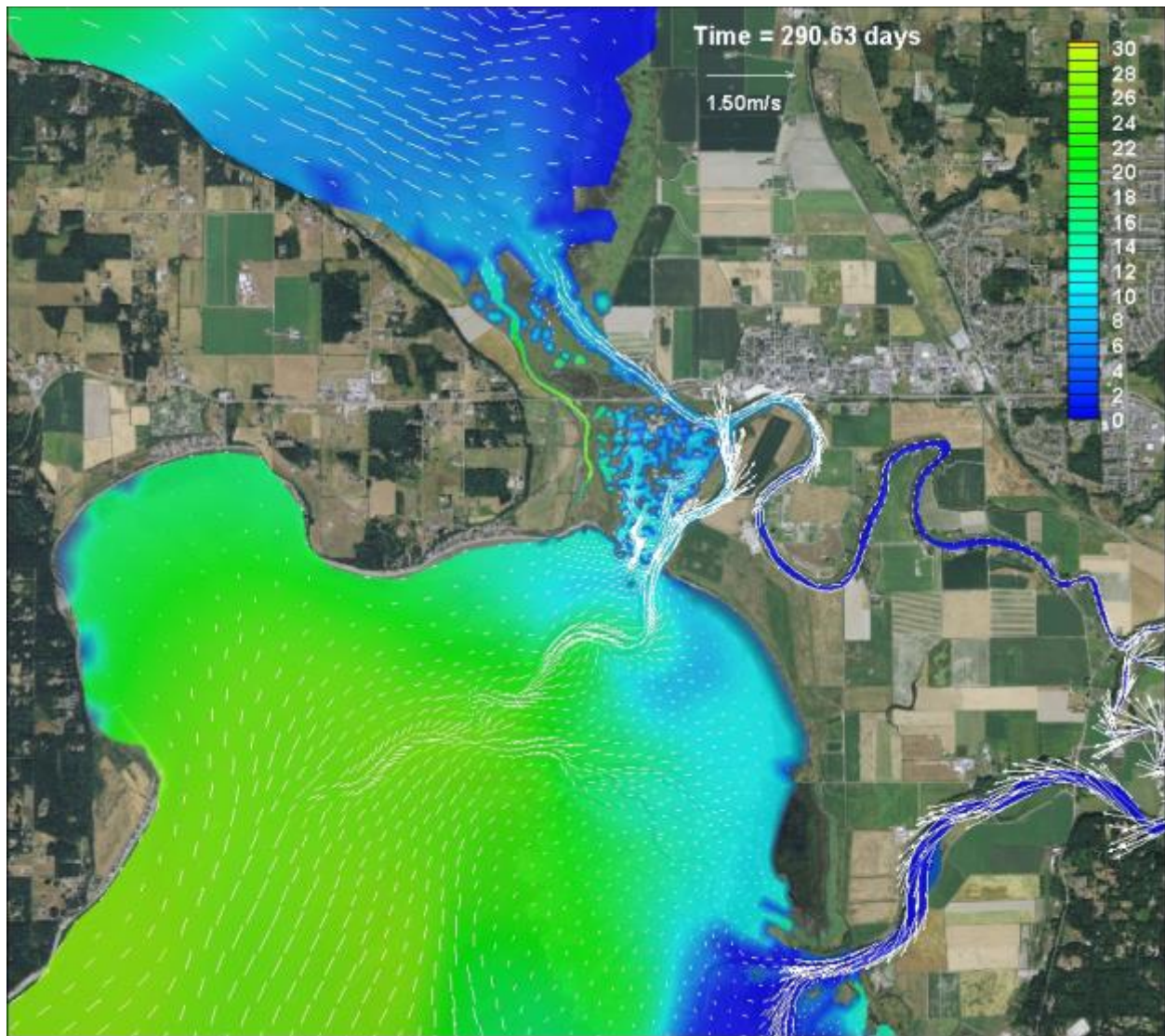
Figure B-16: Scenario 3 (Full Restoration Leque 1) – Salinity contours and velocity vectors, October 17, 2005, peak flood
