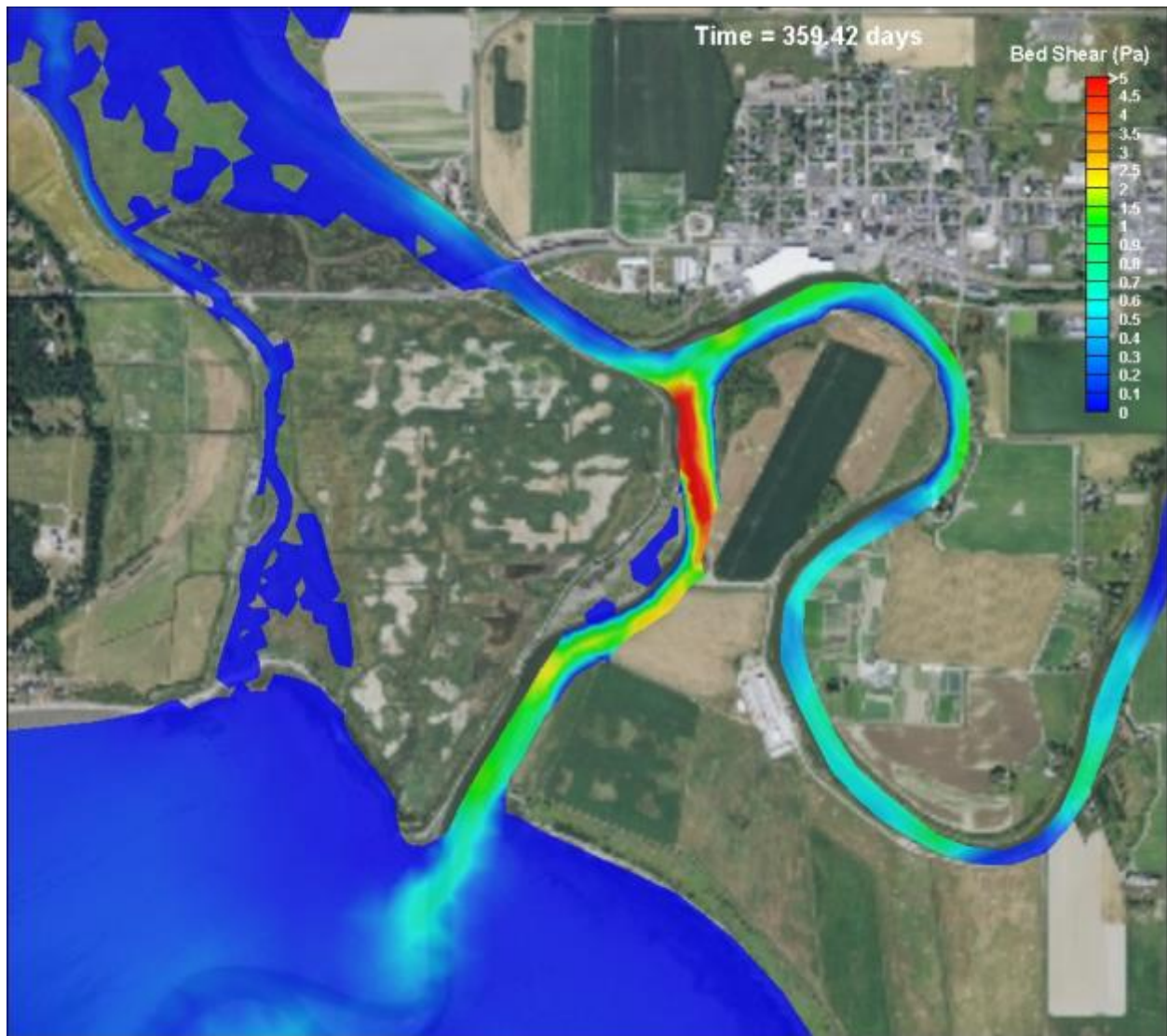
Figure H-19: Scenario 0 (Baseline Condition) – Bed shear, maximum tide during year-long simulation based on December 25, 2003
