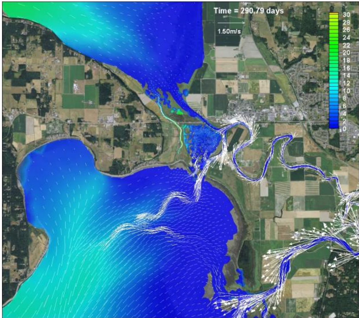
Figure D-11: Scenario 2 (4 Levee Breach Leque) – Salinity contours and velocity vectors, high flow (full bank) condition at 26,508 cfs and peak ebb based on October 17, 2005
