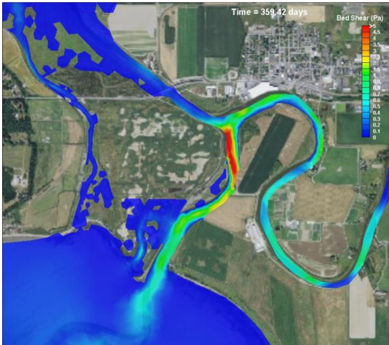
Figure H-20: Scenario 1 (Partial Restoration Leque) – Bed shear, maximum tide during year-long simulation based on December 25, 2003
