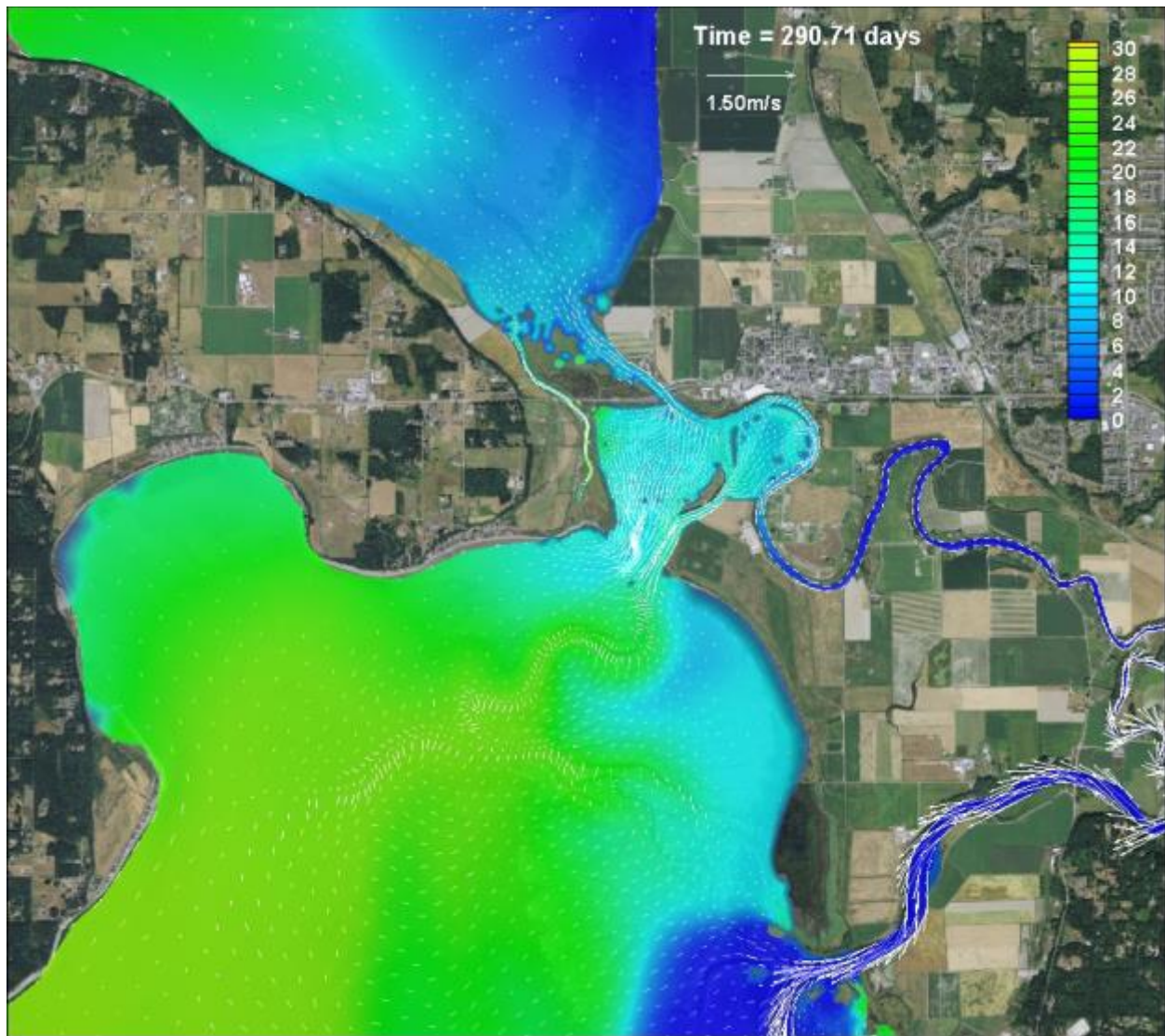
Figure B-29: Scenario 7 (Full Restoration zis a ba + SCN3) – Salinity contours and velocity vectors, October 17, 2005, high tide
