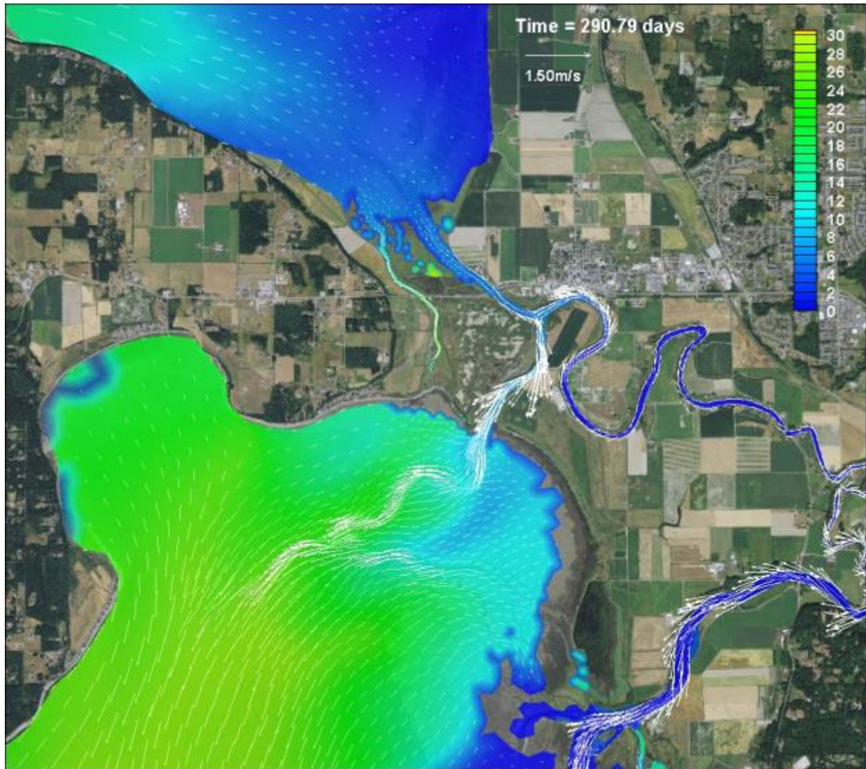
Figure B-3: Scenario 0 (Baseline Condition) – Salinity contours and velocity vectors, October 17, 2005 peak ebb
