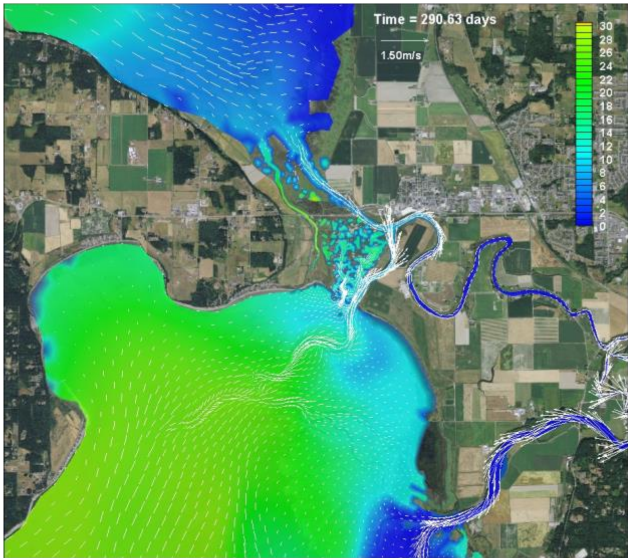
Figure B-20: Scenario 4 (Full Restoration Leque 2) – Salinity contours and velocity vectors, October 17, 2005, peak flood
