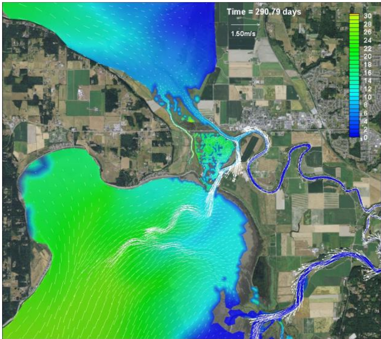
Figure B-35: Scenario 8 (3 Levee Breaches Leque) – Salinity contours and velocity vectors, October 17, 2005, peak ebb
