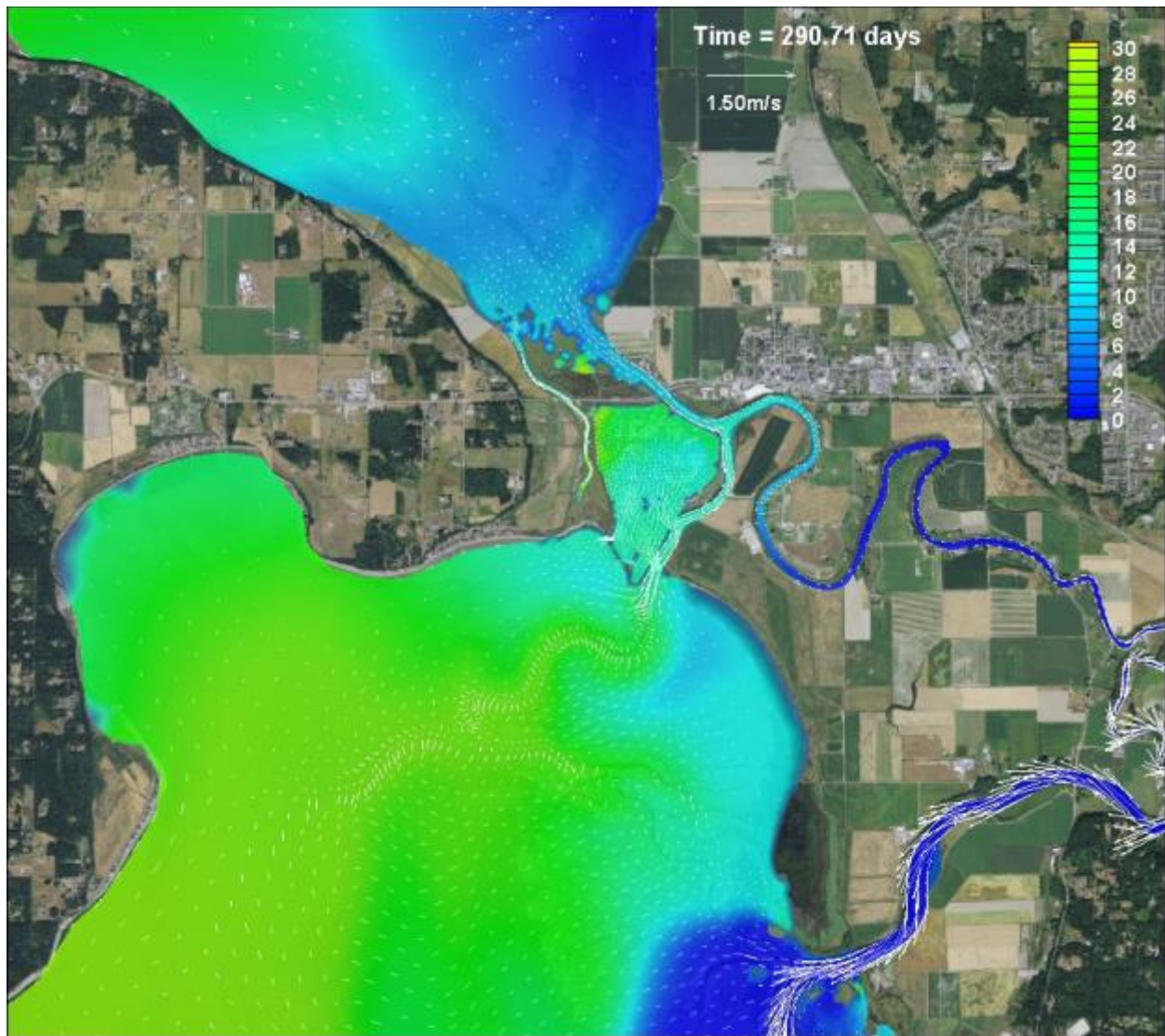
Figure B-33: Scenario 8 (3 Levee Breaches Leque) – Salinity contours and velocity vectors, October 17, 2005, high tide
