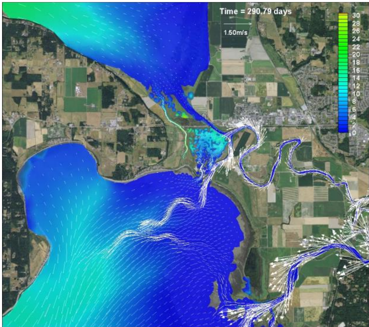
Figure D-19: Scenario 4 (Full Restoration Leque 2) – Salinity contours and velocity vectors, high flow (full bank) condition at 26,508 cfs and peak ebb based on October 17, 2005
