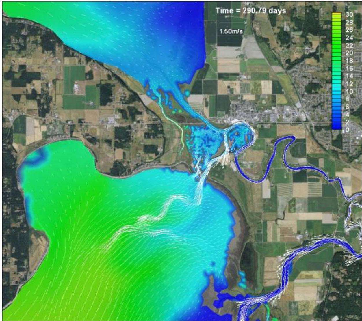
Figure B-31: Scenario 7 (Full Restoration zis a ba + SCN3) – Salinity contours and velocity vectors, October 17, 2005, peak ebb
