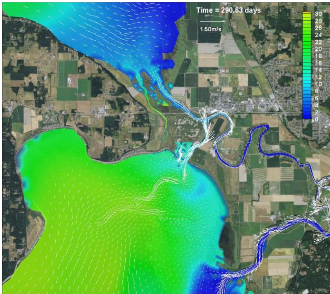
Figure B-8: Scenario 1 (Partial Restoration Leque) – Salinity contours and velocity vectors, October 17, 2005, peak flood
