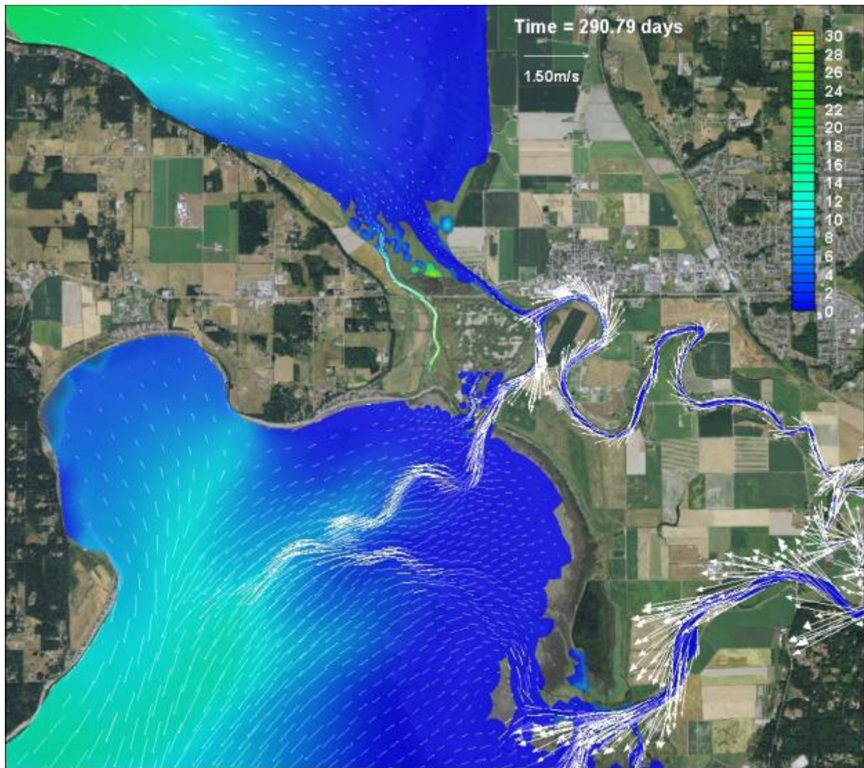
Figure D-7: Scenario 1 (Partial Restoration Leque) – Salinity contours and velocity vectors, high flow (full bank) condition at 26,508 cfs and peak ebb based on October 17, 2005
