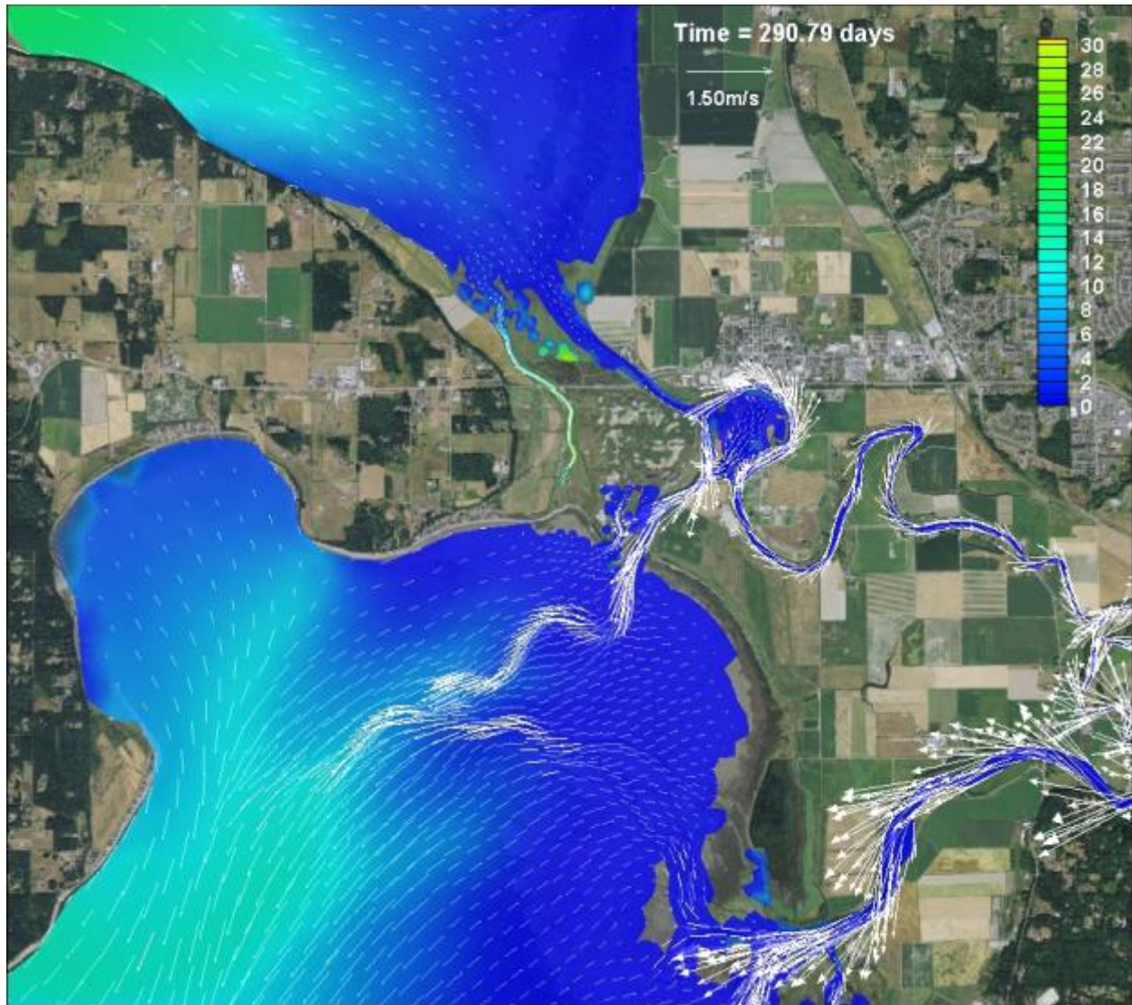
Figure D-23: Scenario 5 (Full Restoration zis a ba + SCN1) – Salinity contours and velocity vectors, high flow (full bank) condition at 26,508 cfs and peak ebb based on October 17, 2005
