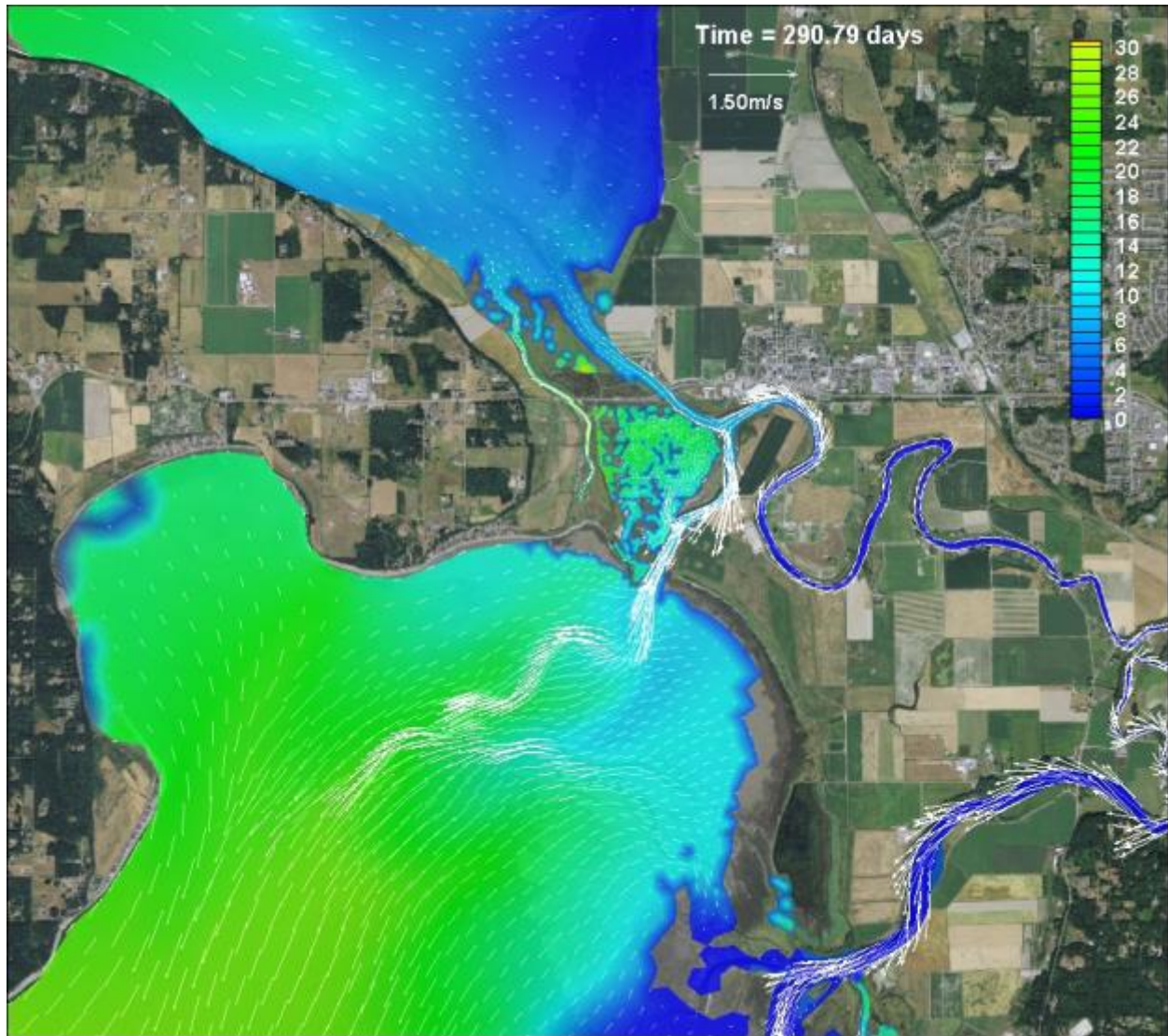
Figure B-11: Scenario 2 (4 Levee Breach Leque) – Salinity contours and velocity vectors, October 17, 2005, peak ebb
