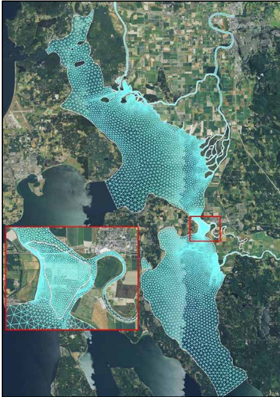
Figure 2-1: Model Grid for Leque Island, Including Skagit Bay and Port Susan Bay and bathymetry
