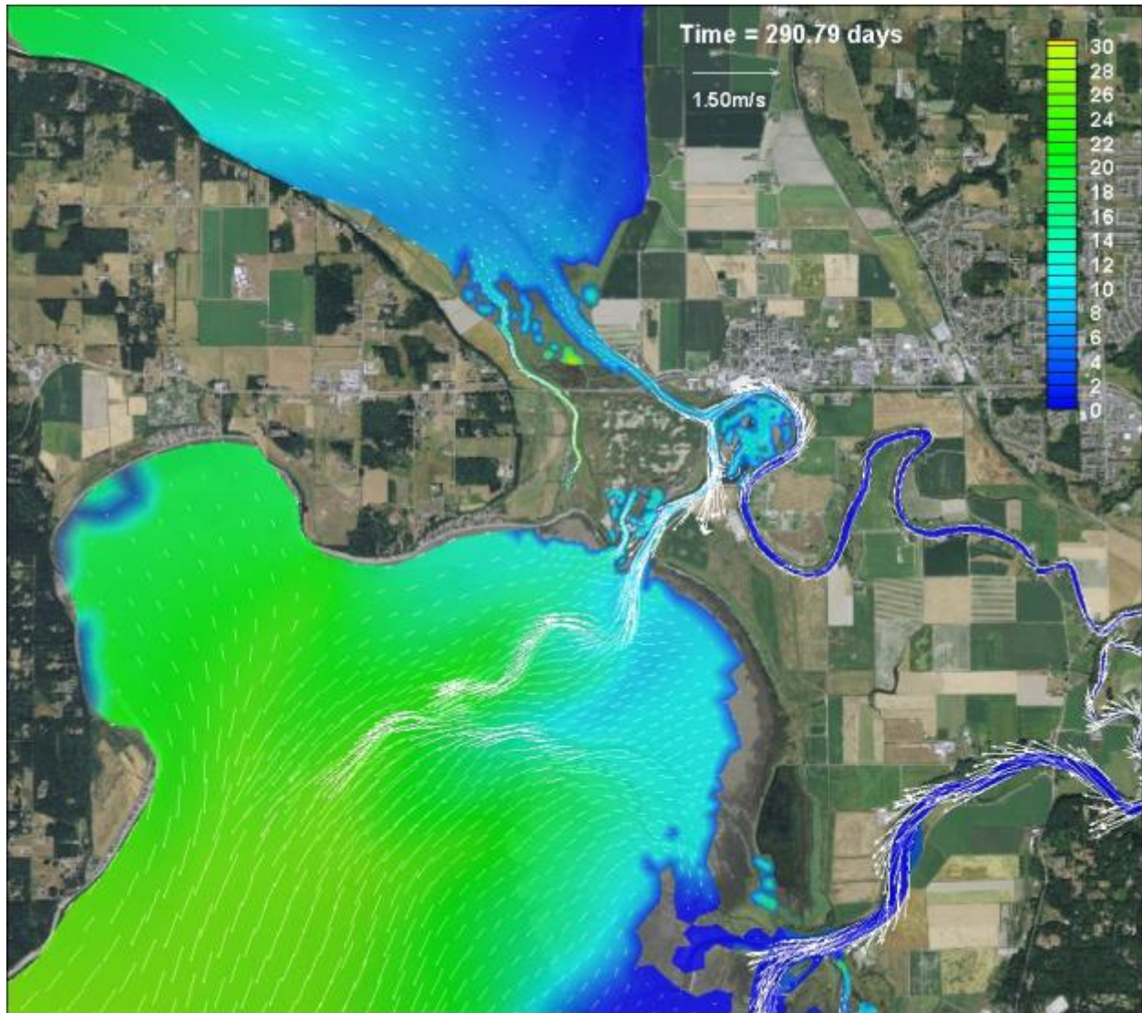
Figure B-23: Scenario 5 (Full Restoration zis a ba + SCN1) – Salinity contours and velocity vectors, October 17, 2005, peak ebb
