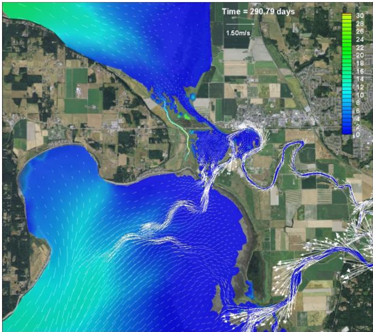
Figure D-31: Scenario 7 (Full Restoration zis a ba + SCN3) – Salinity contours and velocity vectors, high flow (full bank) condition at 26,508 cfs and peak ebb based on October 17, 2005
