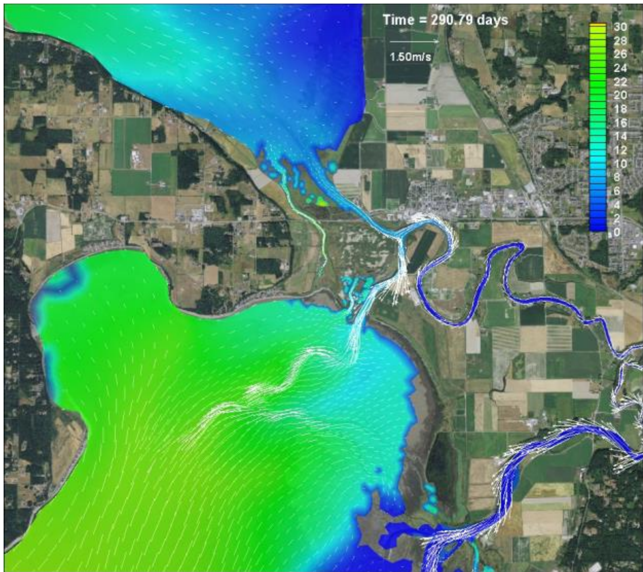
Figure B-7: Scenario 1 (Partial Restoration Leque) – Salinity contours and velocity vectors, October 17, 2005, peak ebb
