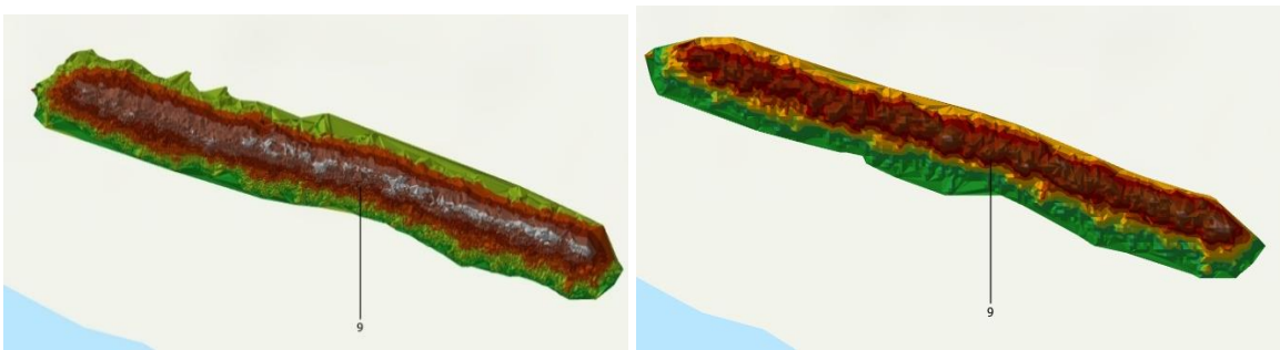
Figure 29. These two images show the results of the LiDAR scans at breakwater unit #9 located at the eastern end of the breakwater project area. The left image is of the “As Built” post construction scans and shows the unit was relatively consistent in elevation and width across the structure with slightly higher elevations seen along the mid-section and eastern side of the crest. The image on the right is the one-year post construction scan. The unit shows signs of settlement in crest elevations across the structure but remains within anticipated ranges and in fully functional condition. These scans do not reveal any scattering of stone with little deformation of the overall configuration. The minor elevation loss appears to be related to settlement rather than wave impact deformation.
