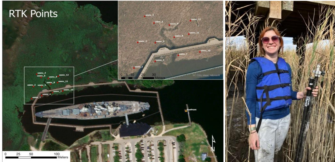
Figure 4. Map of the twelve permanent 1m 2 -quadrats within our Phragmites australis -dominated reference marsh (left), and Danielle Jenkins, a recent graduate of the Master of Marine Science Program at UNCW and continuing member of the Eulie lab, posing within the reference marsh with the survey poles used to collect GPS and elevation of our quadrats.
