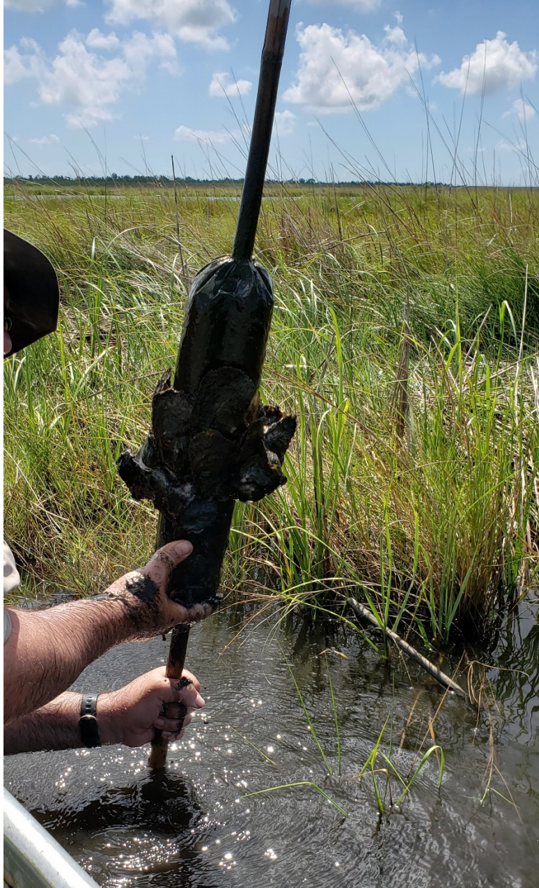
Figure 22. An Oyster Stake with oysters only growing on the middle region of the settlement substrate on 1 June 2022, Golden Meadow site. The lower end of the settlement substrate had submerged or was buried by sediment and the upper end of the settlement substrate may have been exposed at low tide thus preventing oyster and barnacle settlement and growth.
