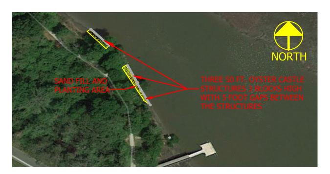
OYSTER CASTLE BLOCKS STACKED 3 WIDE, 3 HIGH WITH 5 FOOT GAPS BETWEEN EACH 50 FOOT SECTION. SAND FILL WITH SAND BROUGHT TO SHORELINE WITH BOBCAT, THEN HAND PLACED WITH WHEELBARROW.
