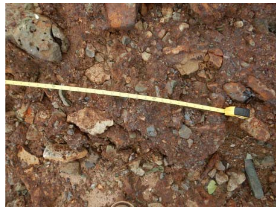
079 - Cemented iron-sand-cobble-slag conglomerate found along shoreline of project site. Location 8.
