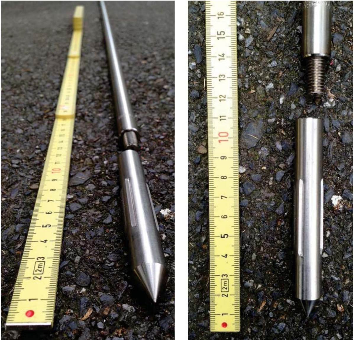
Figure 3.2. Stainless steel rod showing the driving point used on the first rod. Note the threaded studs used to couple sections of rod together.
