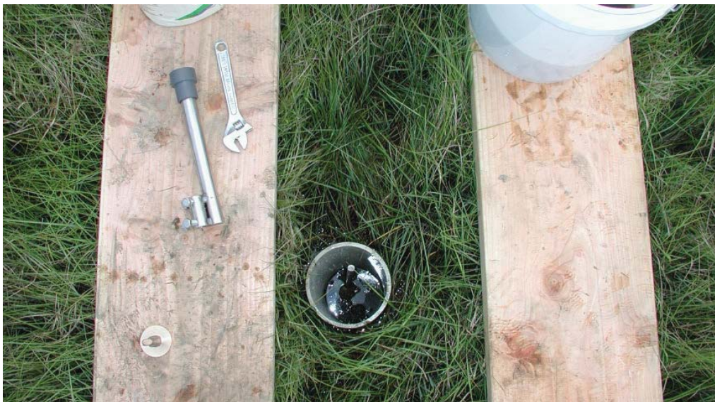
Figure 3.21. Receiver (on wooden plank) prior to attachment to the deep SET mark.
