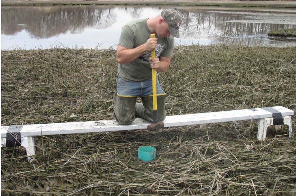
Figure 3.20. Installing the PVC collar (Boston Harbor Islands NRA, MA USA).
