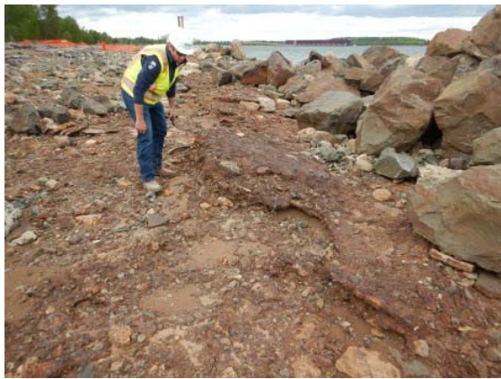
075 - Cemented iron-sand-cobble-slag conglomerate found along shoreline of project site. Location 8.
