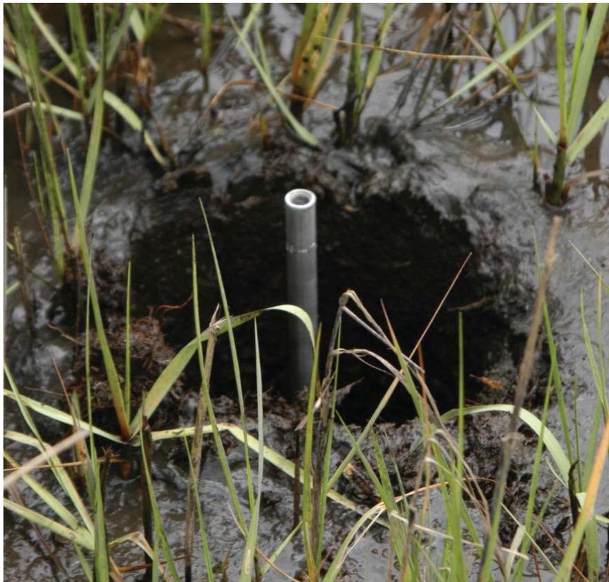
Figure 3.14. Deep SET mark in the hole after pounding has stopped. Note that pounding was stopped at a joint.
