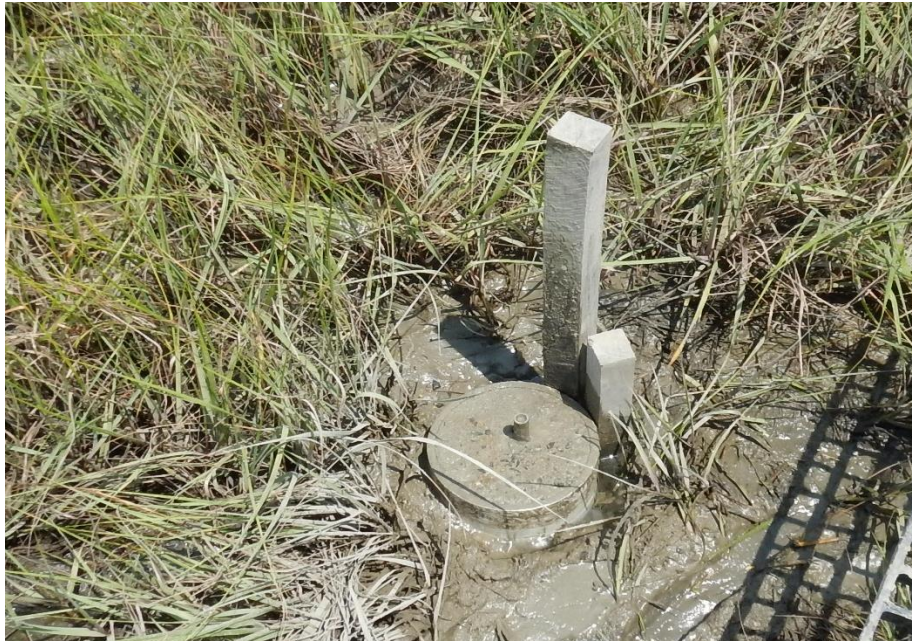
Figure 4: Rod with PVC "collar" filled with cement
