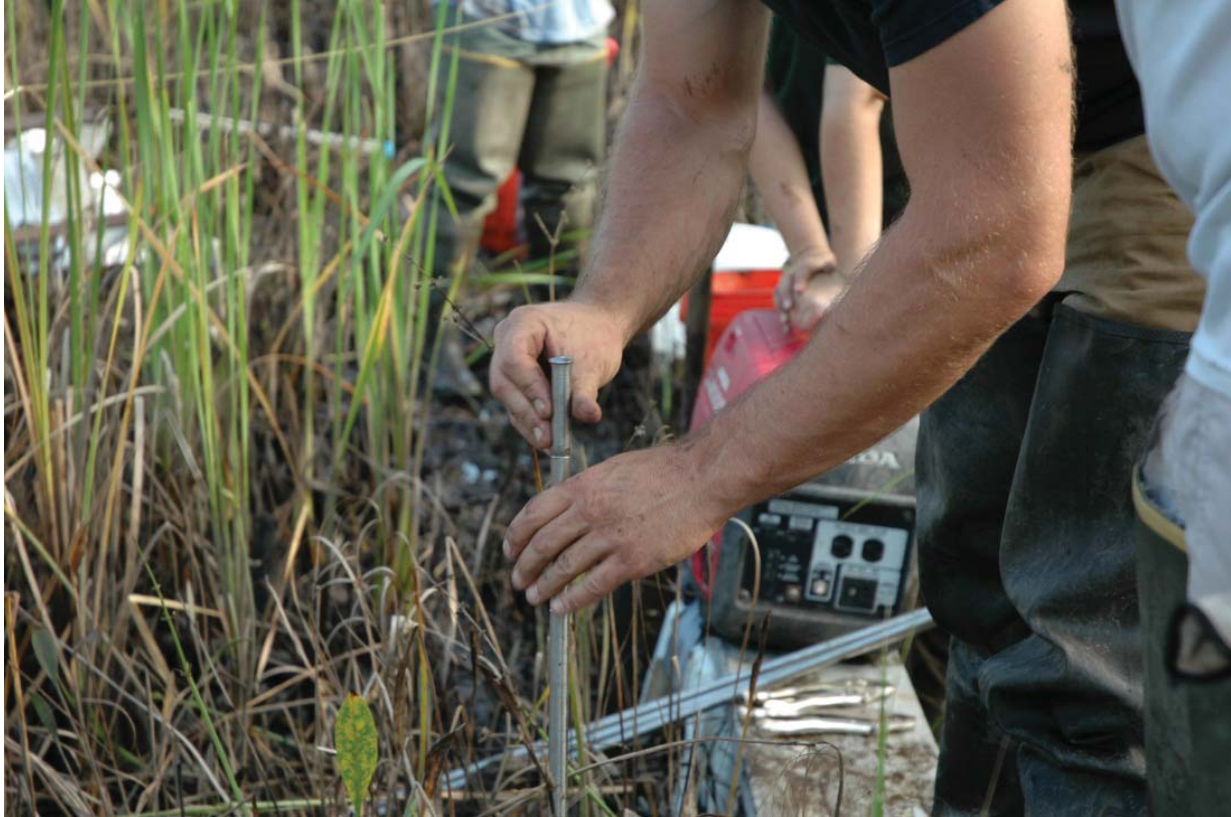
Figure 3.10. Attaching the driving head (Waccamaw River, South Carolina, USA).
