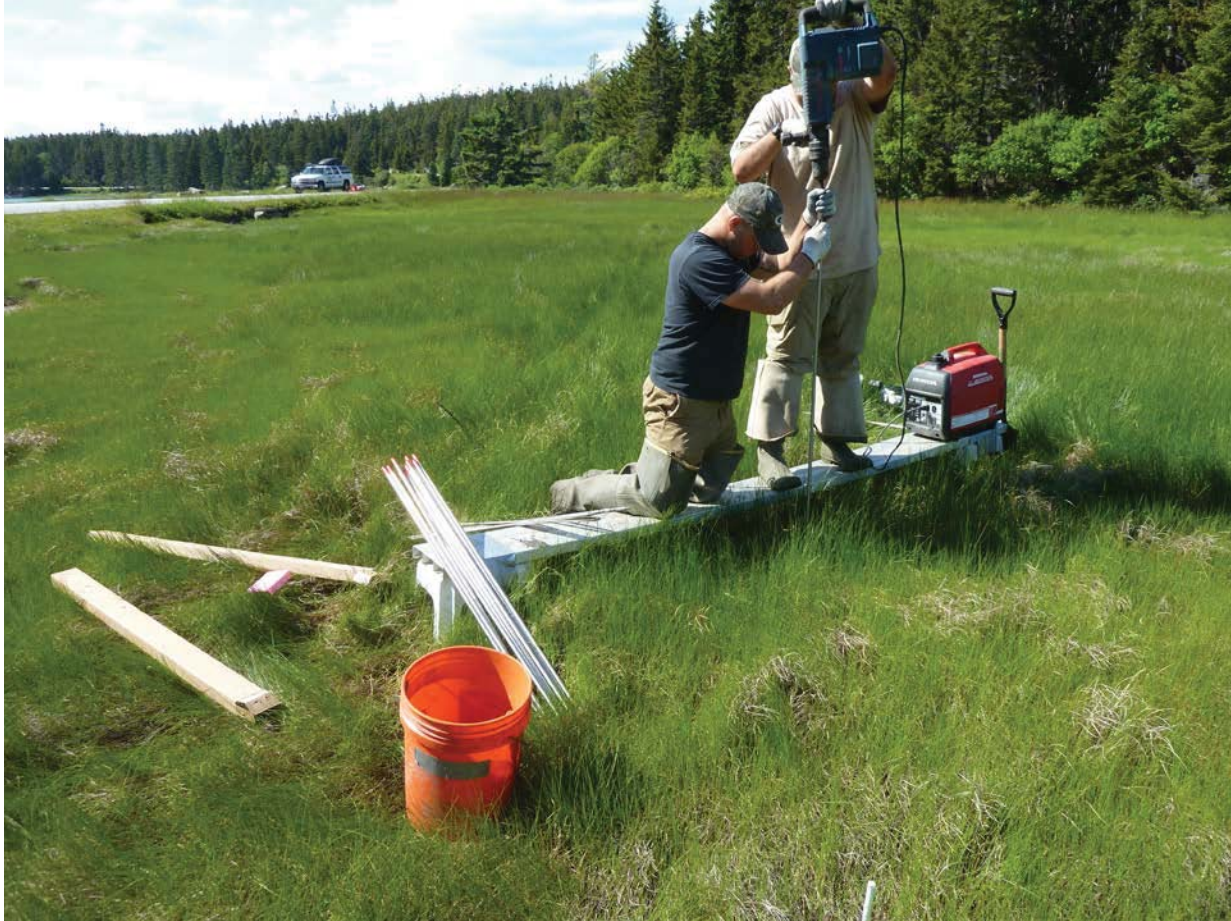
Figure 3.12. Driving rods. Note the bundle of rods on the end of the platform (Acadia NP, ME USA).
